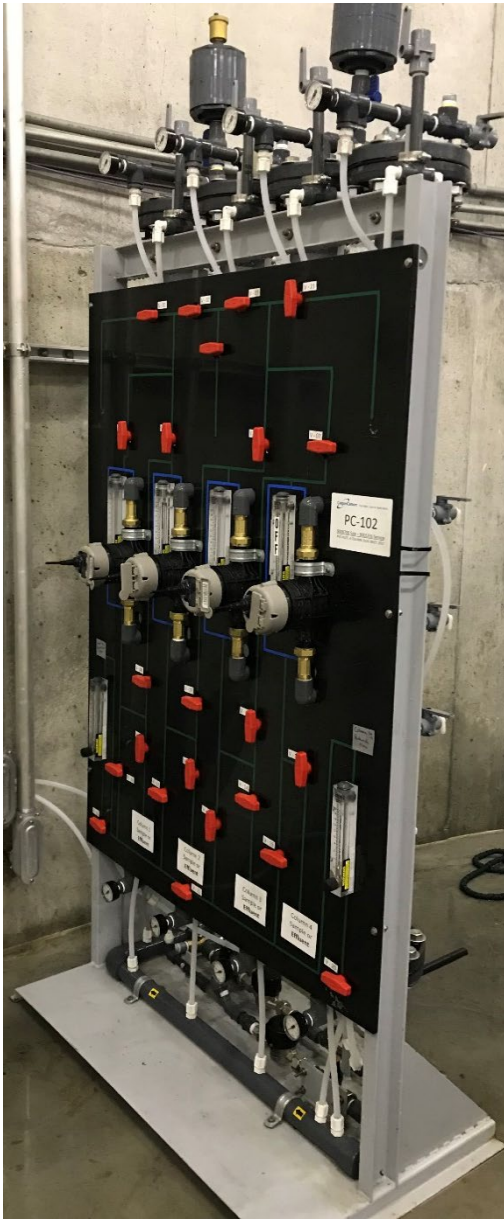
Figures 1 & 2: Photos of front and rear of pilot unit showing 4 columns, flow meters, and interconnecting piping.
